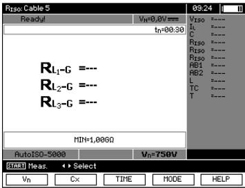
The meter is ready for measurement. Value of interference voltage can be read on the display.
