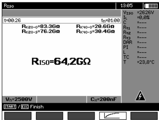
**RK20-O** –  $R_{ISO}$  converted to a value at 20°C for oil insulation (applies i.e. to insulation in **cables**).
