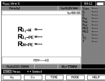
Use **F1** **Vn**, **F2** **Cx** and **F3** **TIME** buttons to adjust the desired test voltage, the capacity of the object, and the measurement time. (Similarly as in section 3.2.2)
