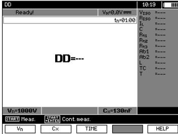
Use **F1** **Un**, **F2** **Cx** and **F3** **TIME** buttons to adjust desired test voltage, capacitance of the object and measurement time (1 min to 60 min), similarly as in section 3.2.2
