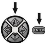
Use **↑**, **↓** to switch on/off the function of Auto-incrementing of the memory cell number. Confirm your choice by pressing **ENTER**.
