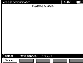
Turn the keyboard on and set it in pairing mode (via a special button on the keyboard – please refer to the manual of the keyboard). Select "F1 – Search" on the meter. The meter will search for available Bluetooth devices; the time to find Bluetooth devices depends on the number of available devices within range.
