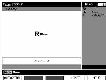
The meter is ready for measurement. Press **F4** **LIMIT** to set the maximum resistance value.
