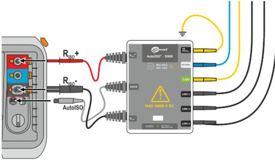
Connect AutoISO-5000 adapter. The meter detects automatically and changes the screen appearance.
