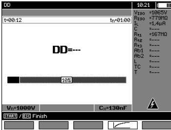
Either during, or after the measurement, the user can switch between the text display of the results and the chart by pressing **F4**
