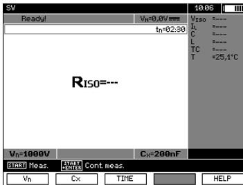
Use **F1** **Vn**, **F2** **Cx** and **F3** **TIME** buttons to adjust desired test voltage, capacity of the object and measurement time, similarly as in section 3.2.2
