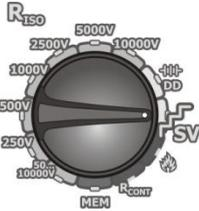
Set the rotary switch of function selection in the **SV** position. The meter is in the voltage measurement mode.
