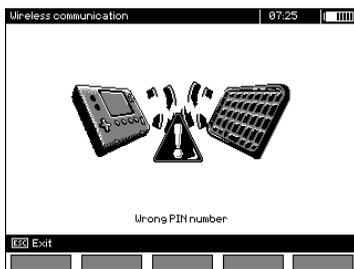
– Wireless connection error Device not found – the keyboard is not available for connection.
