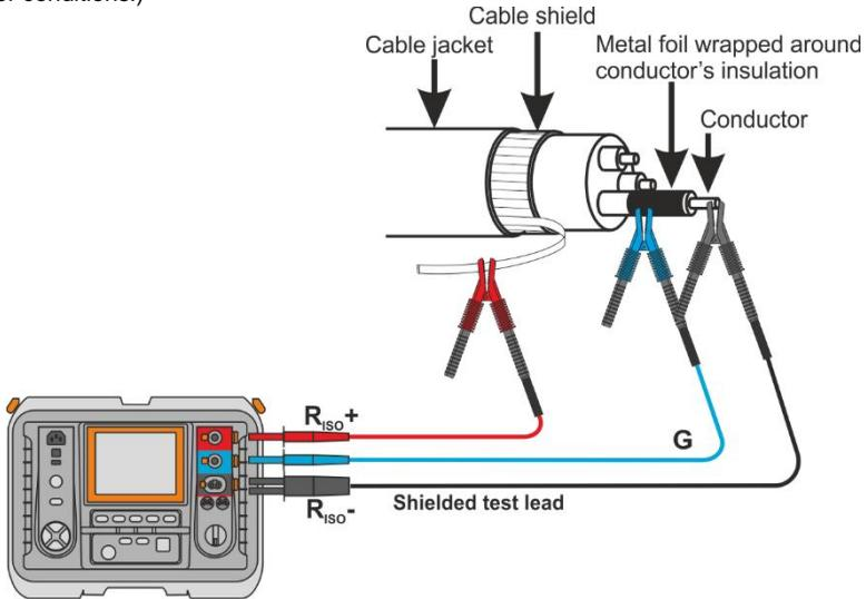
The same method applies when measuring the resistance between two conductors of the cable; attaching the foil to the **G** terminal to ignore other conductors that do not take part in the measurement.
