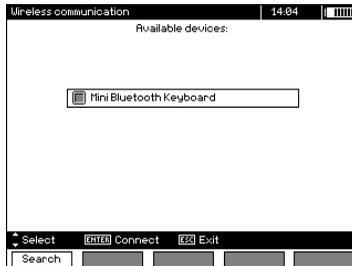
From the list of available devices select a keyboard and press "ENTER -Connect" – the meter will display the progress bar, and a counts of 30 seconds. During this time use the keyboard to enter a PIN code and confirm it by pressing "ENTER".
