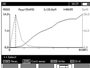
Use **←**, **→** to move the vertical dashed cursor line to display measurements at a selected time. The display will show data for measured values at the point where the cursor is positioned. The measurement result indicates the status of the insulation. Refer to the following table:
