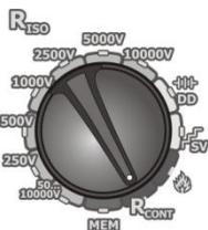
Set the rotary switch at the  $R_{CONT}$  position.
