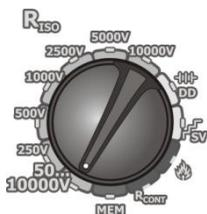
Set the rotary function selection switch at the position of a chosen  $R_{ISO}$  measuring voltage. The voltage is adjusted as follows:
