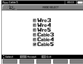
Press **F4** **MODE** button to enter the selection of lead/ cable type (3-, 4- or 5-wire lead).
