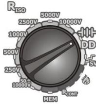
Set the rotary function selection switch at **DD**. The meter is in the voltage measurement mode.
