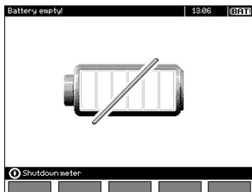
Battery completely discharged. Measurements cannot proceed until battery is recharged.
