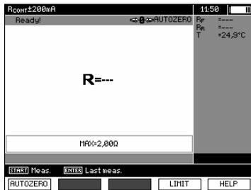
An **AUTOZERO** message appears confirming that calibration of the test leads has been performed. The meter then enters the measurement mode. The **AUTOZERO** message is displayed during measurements. The compensation values are retained even after the meter is switched off and on again.
