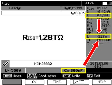
The device measures the total capacity of the cable **C [nF]**. Using this value and when the unit capacity **C<sub>x</sub> [nF/km]** is entered, it may calculate the length **L**.
